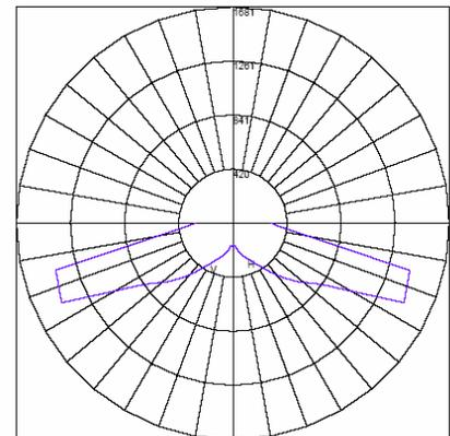
Maximum Candela = 1651 Located At Horizontal Angle = 65, Vertical Angle = -37.5
